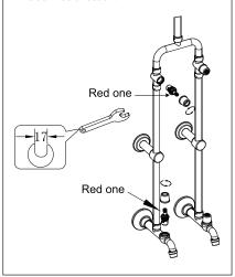
4. Insert BLUE cartridge. Tighten the cartridge by using spanner in clockwise direction, tighten the cartridge cover plate in clockwise direction.
