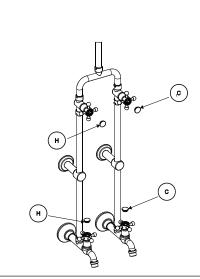
2. Remove the screws by using a screwdriver in anti-clockwise direction, then remove the cross handles.
