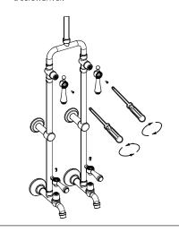
**6.** Attach the H Cover plate on the Left and the C cover plates on the right.
