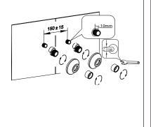
3. Use the measurements shown to mark out the 3 fixing points on the wall to attach the 3 connectors (12). Drill the 3 holes at the fixing points using a 6mm drill bit. Insert the plastic screw plugs into the drilled holes. Using a screwdriver attach the 3 connectors (12) with the screws provided.
