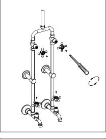
3. Remove the left cartridge cover plate turning anti-clockwise, then take out the RED cartridge by using a spanner in anti-clockwise direction.
