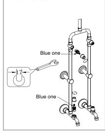
5. Tighten the H cartridge switch anti clockwise. Tighten the C cartridge switch clockwise. Attach the lever handles to the cartridge and tighten the screws by using a screwdriver.
