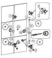
5. Insert 2 filters (5) into the top of the shower taps (7). Attach rail (8) to the shower taps by screwing the connectors clockwise. Insert filter (5) into the top of rail (8). Attach rail (9) to rail (8) by screwing the connector clockwise. Put cover plate (10) over the connector at the top fixing point on the wall. Using a screwdriver tighten the wall bracket to the rail with screw (11). Put the wall bracket over the top fixing point connector and tighten the grub screw with the Allen key.
