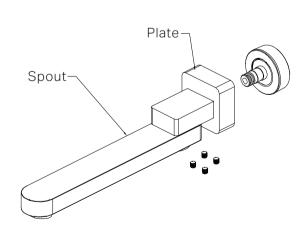
4. Insert the spout and tighten the four grub screws.
