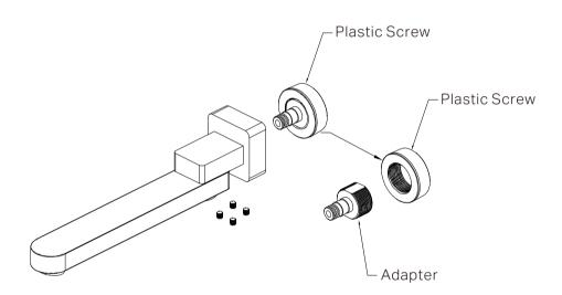
2. Unscrew the grub screws, and unscrew the adapter and plastic screw.
