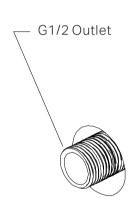
1. Ensure that the G1/2 outlet thread is less than 14mm, trim the outlet if necessary to achieve the desired fit. Apply the G1/2 water outlet connection with Teflon tape to ensure a watertight seal.
