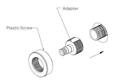
3. Screw the adapter and plastic screw in a row.
