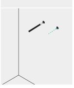
2. Drill pilot holes for the wall anchors where you have marked the location of the mounting screws. Use a drill bit that is slightly smaller than the size of the wall anchors (between 6-8mm).
