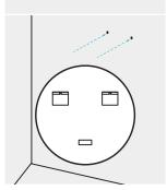
Drill pilot holes for the wall anchors where you have marked the location of the mounting screws. Use a drill bit that is slightly smaller than the size of the wall anchors (between 6-8mm).
